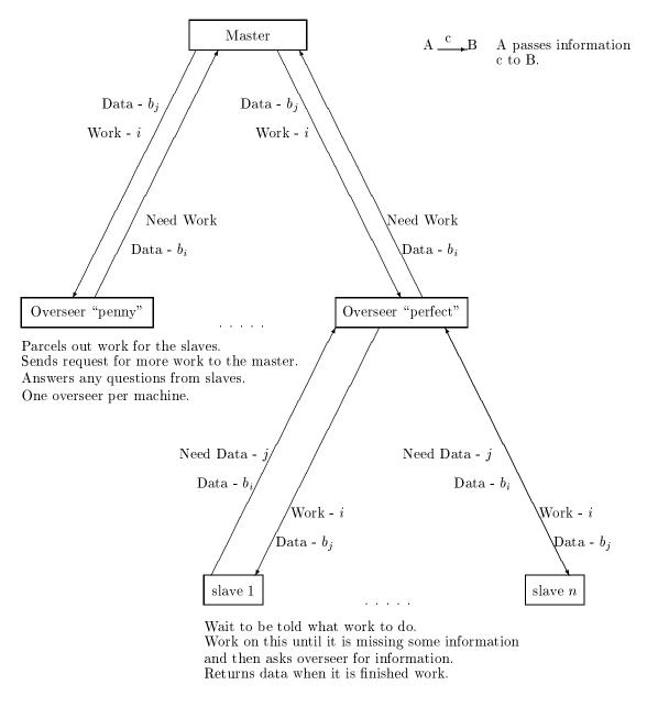
Figure 6.2: Load balancing master/overseer/slave diagram.
